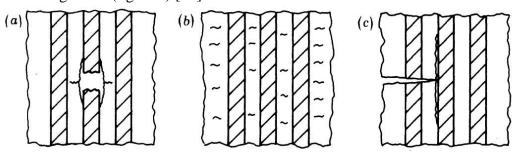
Figure 2. Fatigue damage mechanism in unidirectional composites under parallel loading tofibers: (a)fiber breakage, interfacial debonding; (b) matrix cracking; (c) interfacial shear failure [18]
