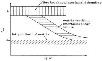
Figure 3.Fatigue-life diagram for unidirectional composites under loadingParallel to fibers [18].
