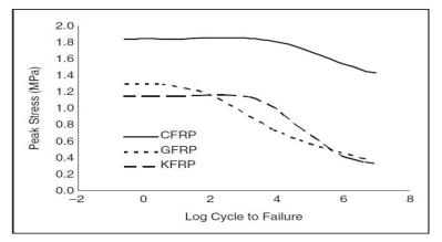
Figure 1. S-N curve for unidirectional Composite materials [14].
