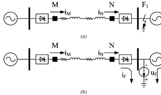
Fig. 3. External fault at the inverter side considering the series inductance of the dc transmission line
