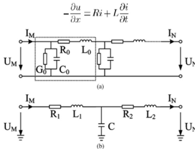
Fig. 2. Demonstration of line models. (a) Distributed parameter model
