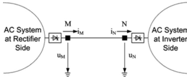
Fig. 1. Diagram of the HVDC transmission system
