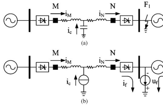
Fig. 4. External fault at the inverter side considering the shunt capacitance of the dc transmission line
