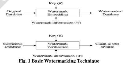
In watermark embedding, a private key K, which is only known to the owner, is used to embed watermark W into the original database then the output of these phase is publically available. The verification is performed to verify the ownership of suspicious database. In this phase, suspicious database is taken as input and with the help of private key K the embedded watermark is extracted. Figure 1 shows the basic database watermarking technique [2].
