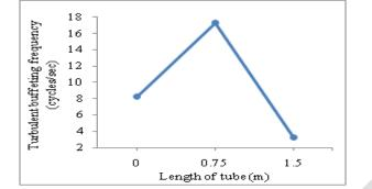
Figure 5: Turbulent Buffeting Frequency vs length of tube
