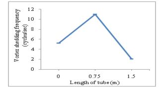
Figure 4: Vortex shedding frequency vs length of tube
