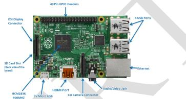
Figure 2. Raspberry Pi B+ model Diagram
