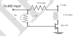
Figure 1. Signal conditioning circuit
