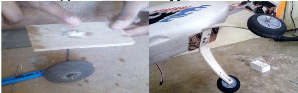
(Figure 7.8: Construction and installation of landing gear)
