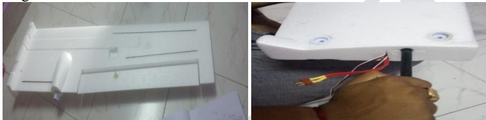
(Figure 7.2: place of carbon strip and insert the carbon tube in the wing)
