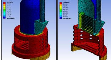
Figure No. 4: Temperature Distribution Analysis of Boiler.
