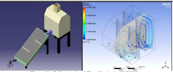
Figure No. 7: Designed and Flow Simulation of Dryer.
