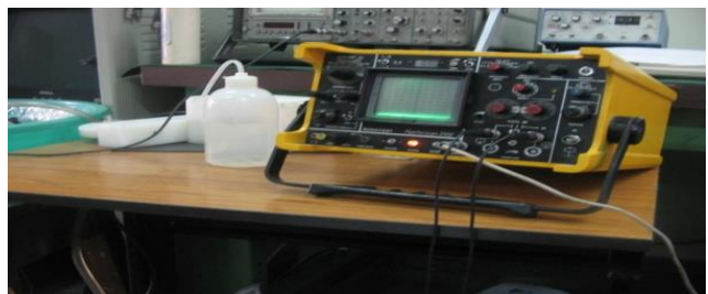
Pulse-Echo test experimental set up
