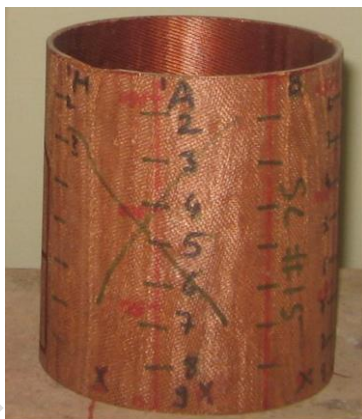
High Silica Phenolic Through Transmission experimental set up
