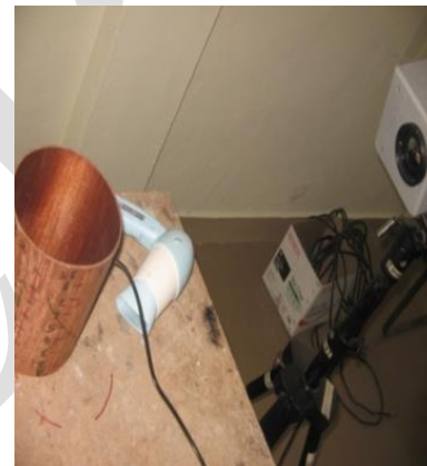
High Silica Phenolic Through Transmission experimental set up
