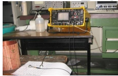
Through Transmission test experimental set up
