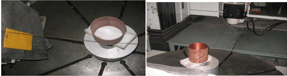
Tangential Radiography experimental set up
