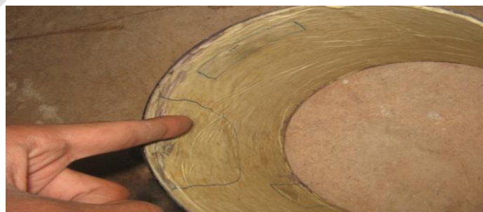
EPDM rubber bonded inside to Maraging steel casing
