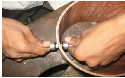
Through Transmission test experimental set up
