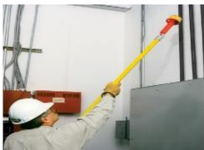
Fig. No. 4 New High Voltage Indicator
