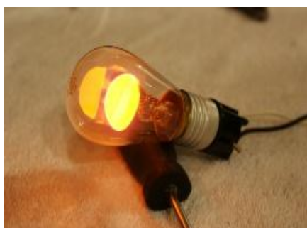
Fig. No.3 Old High Voltage Indicator
