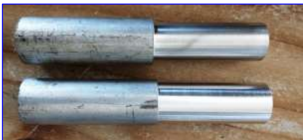
Fig 4. Work- piece after machining
