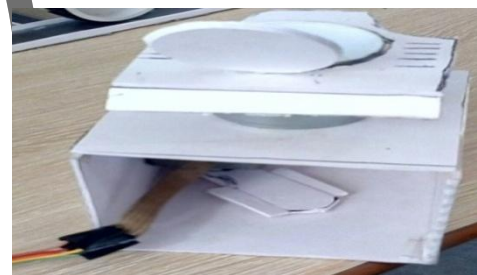
Fig .no.14. locked position of lavatory pipe
