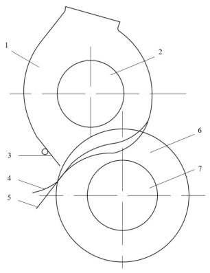
Figure 1. Schematic of a 5LP linter working chamber with EN profile and improved construction
