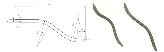
Figure 2. Drawing of 5LP linter column with improved design (a. Simple design, b. Improved design)
