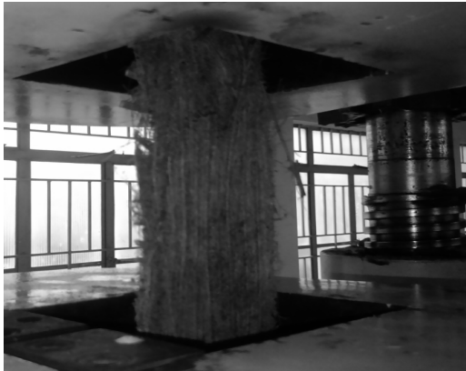
Fig. 3 Biocomposite specimen tested on UTM
