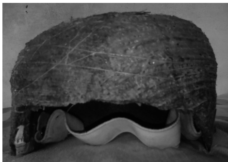
Fig. 7 Coir Fiber Biocomposite Helmet for Child
