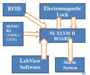
**LabVIEW:** LabVIEW is a graphical programming language that uses icons instead of lines of text to create applications. In contrast to text-based programming languages, where instructions determine program execution, LabVIEW uses dataflow programming, where the flow of data determines execution.
