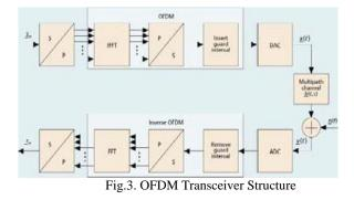
Fig.3 shows the configuration for a basic OFDM Transmitter and Receiver. The signal generated is at base band and so to generate an RF signal, the signal must be filtered and mixed to the desired transmission frequency.
