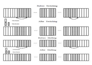
Fig. 4 Null Subcarriers Switching/ Shifting technique for PAPR reduction in OFDM signal
