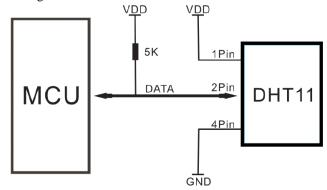
Figure-1. Dht11 connection with the PLC unit or single chip PIC microcontroller
