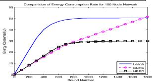
Fig: 7. Comparison of energy consumption rate of LEACH, SCHS and HEED.
